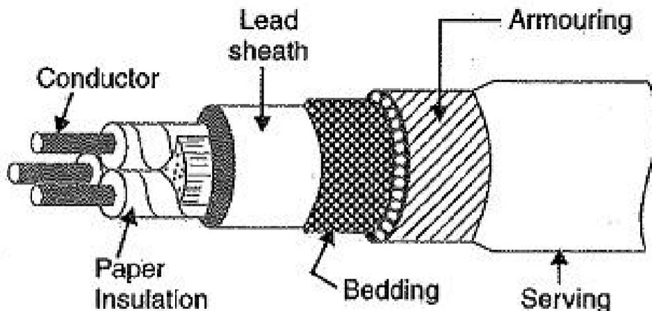
**Fig. 11.1 Construction of a Cable**
