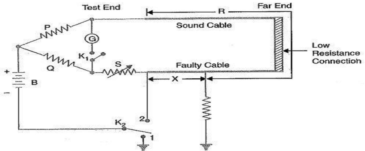
**Fig. 11.24** Varley Loop Test (Earth Fault)
