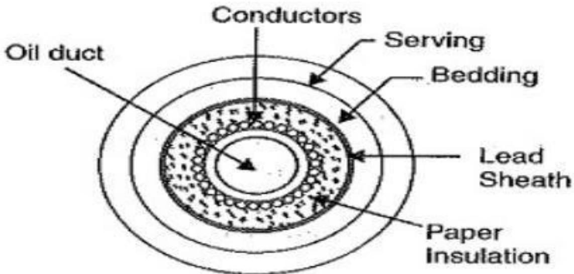
**Fig. 11.6** Single-core conductor channel, oil-filled cable
