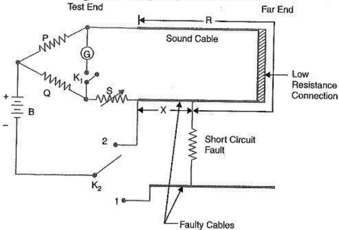
For earth fault or short-circuit fault, the key  $K_2$  is first thrown to position 1. The variable resistance  $S$  is varied till the bridge is balanced for resistance value of  $S_1$ . Then,
