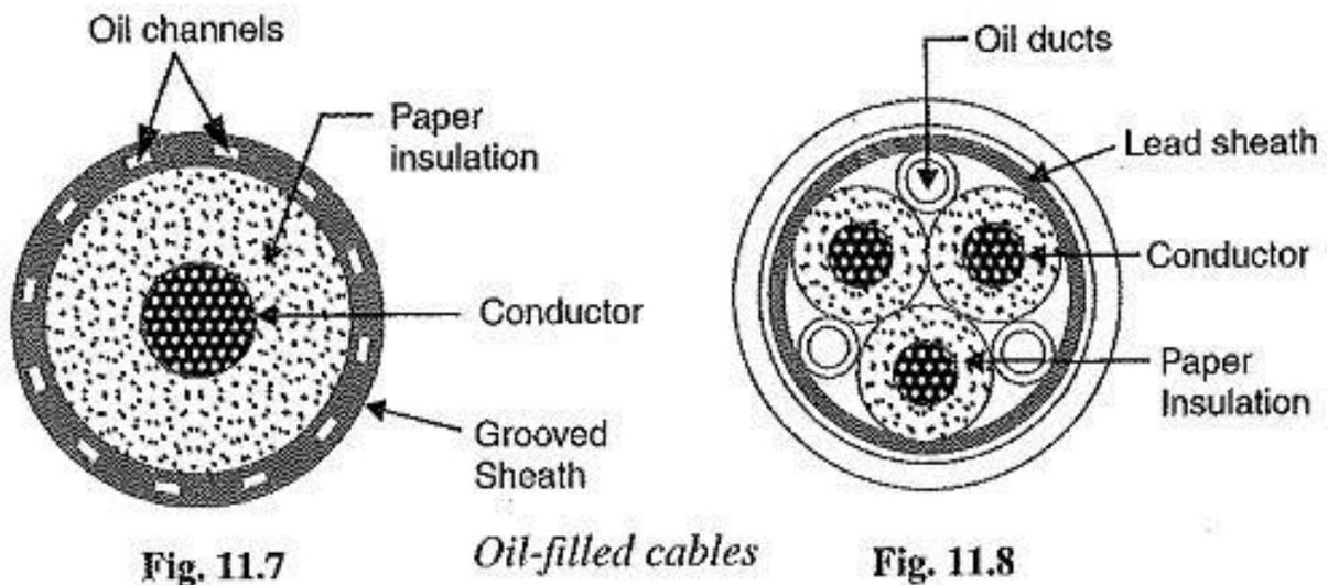
Fig. 11.7 shows the constructional details of a single core sheath channel oil-filled cable. In this type of cable, the conductor is solid similar to that of solid cable and is paper insulated. However, oil ducts are provided in the metallic sheath as shown in Fig. 11.8, the oil ducts are located in the filler spaces. These channels are composed of perforated metal-ribbon tubing and are at earth potential.
