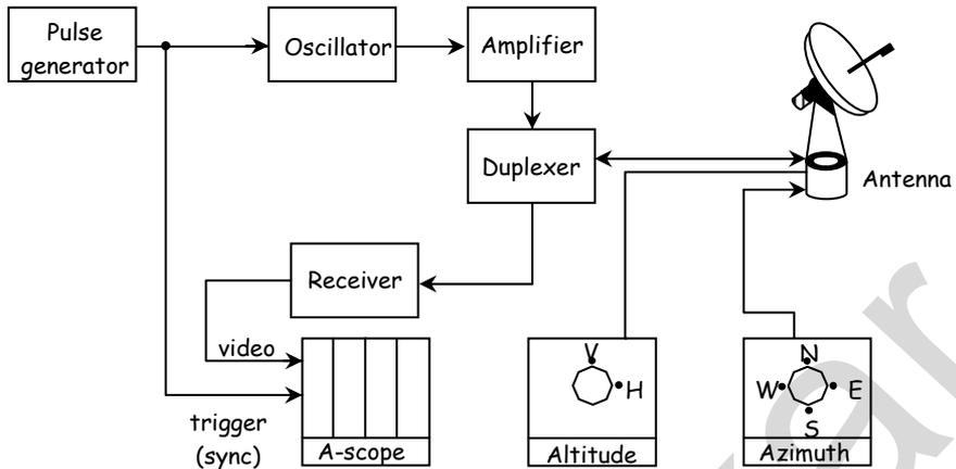
Fig.2 : Block diagram of pulsed radar
