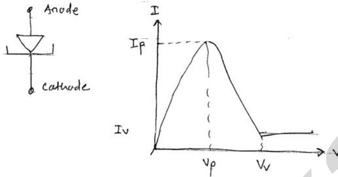
The Tunnel diode is a specially made P-N junction diode which exhibits negative Resistance over part of the forward characteristics. It has extremely heavy doping on both sides of junction and abrupt transition from P-side to the n-side. The Tunneling effect is a majority carrier effect and is consequently very fast.
