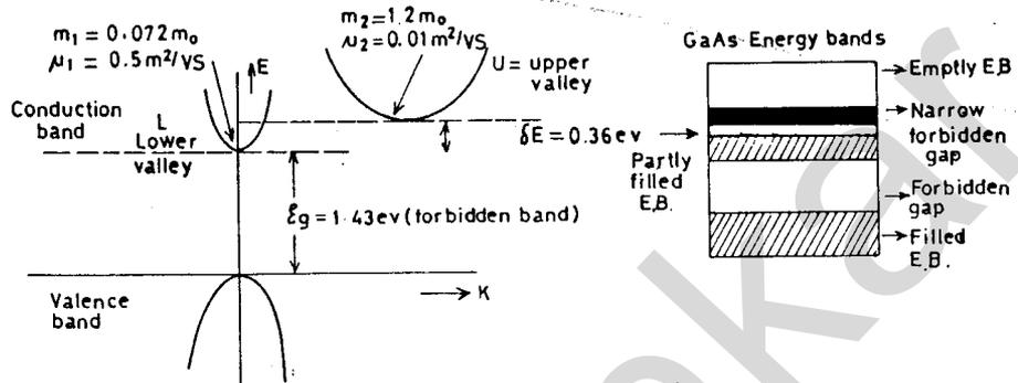
Basic mechanism involved in the operation of bulk n-type GaAs device (gunn diode) is the transfer of electrons from lower conduction valley (L-valley), to upper subsidiary valley (U-valley). This concept of Electron transfer is also known as "Gunn effect".
