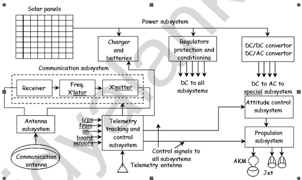
In above figure different subsystem of communication satellite are shown.
