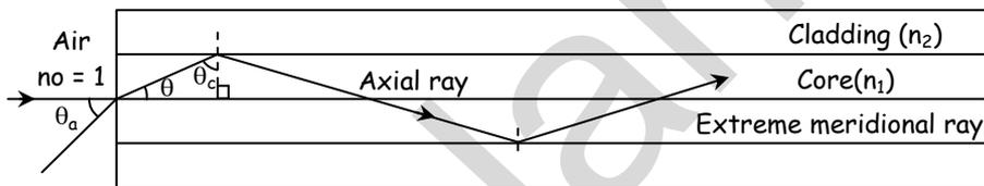
**Fig. 2:** Multimode step index fiber
